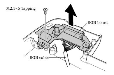
Figure 4-36 Removing the RGB board
